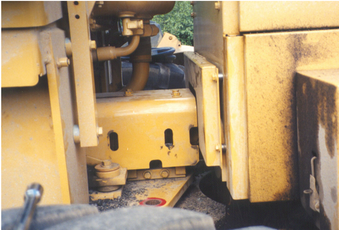
Shields back in place over compressor mount and drive assembly.
