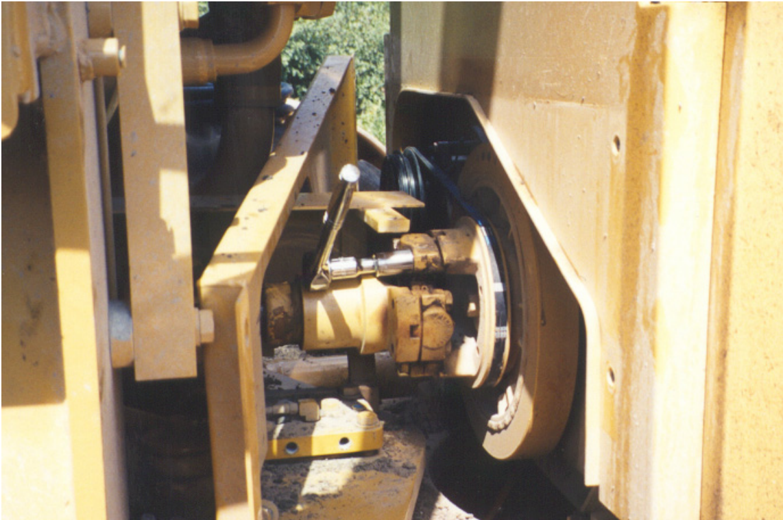
Drive assembly showing drive shaft coupler which must be disconnected to install V-belt.
