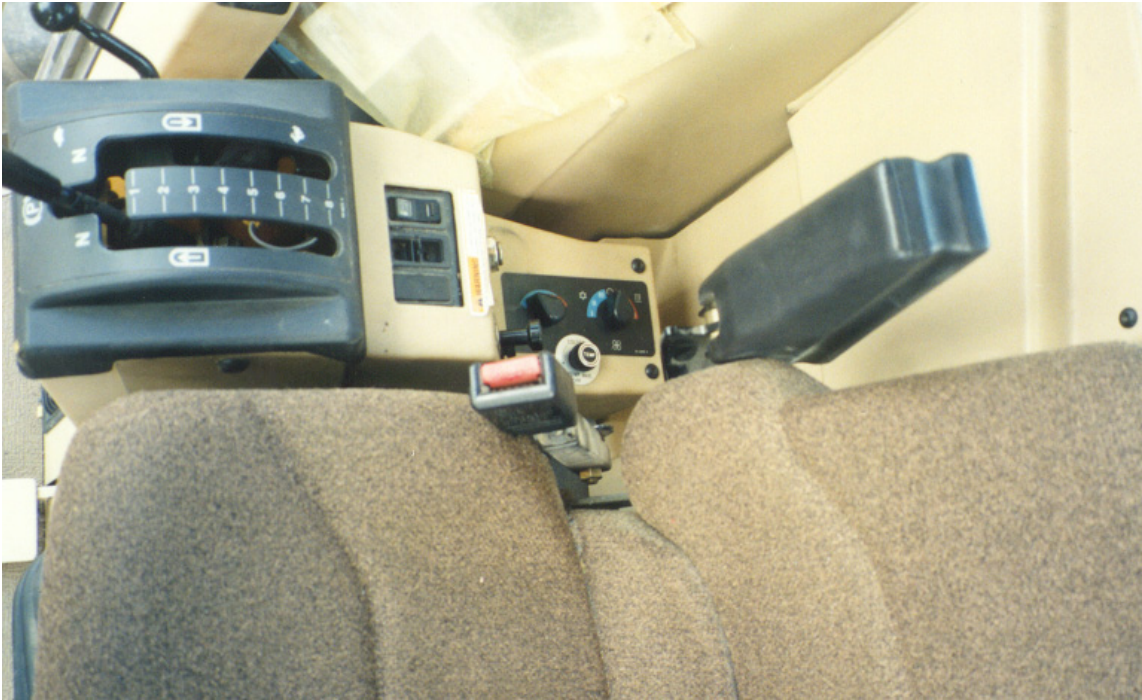
Thermostat in position on control panel.
